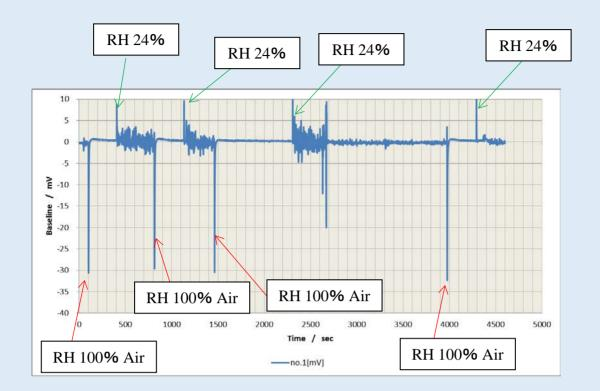
The transient spike response from the sensor for each humidity excursion was of approximately 5s in duration. The results here are expressed in mV from our recommended circuit, with 6mV being equivalent to 1 ppm NO<sub>2</sub>. The maximum amplitude of the spike when the humidity changed from low to high was 5 ppm equivalent, and -1ppm equivalent when humidity was changed from high to low.
