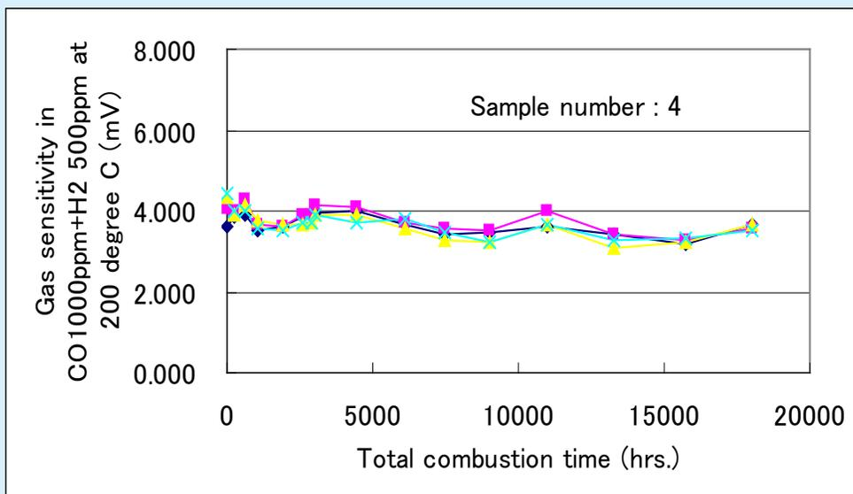
Although the Gas Sensitivity of the sensor does not change significantly during the sensor's lifetime in a real working situation, the zero offset does drift slightly with time. However, this can easily be compensated for in the software of the appliance by carrying out a routine zero correction calibration during periods where the force ventilation of the flue is running but the burner is inactive, ensuring that no combustion gases are in the flue of the boiler during this procedure.
